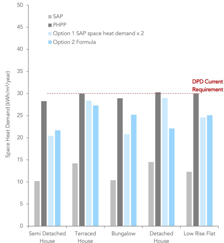
Actual SAP and PHPP space heat demand for homes compliant with the current DPD, compared to the results of two different approaches to produce more realistic values from SAP. Option 1 is simple and can work reasonably well, though Option 2 is expected to more reliably produce results more consistent with PHPP calculations.
