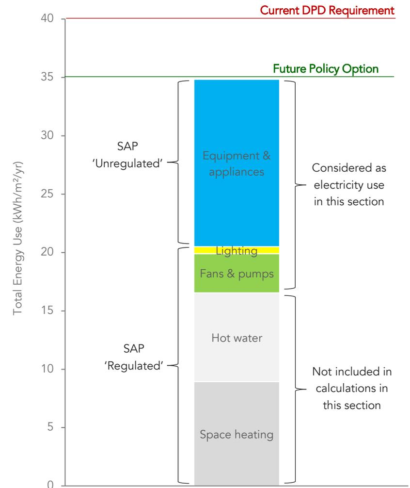
Graph of total energy use for a typical net zero carbon semi-detached house that is compliant with the current DPD policy. This section considers both 'unregulated' energy use and lighting, fans, and pumps, which SAP classes as 'regulated' energy use. PHPP calculates all these energy uses and does not differentiate between them. Note that Equipment and appliances is typically the largest end use of electricity, and is therefore critical to setting total energy use requirements.
