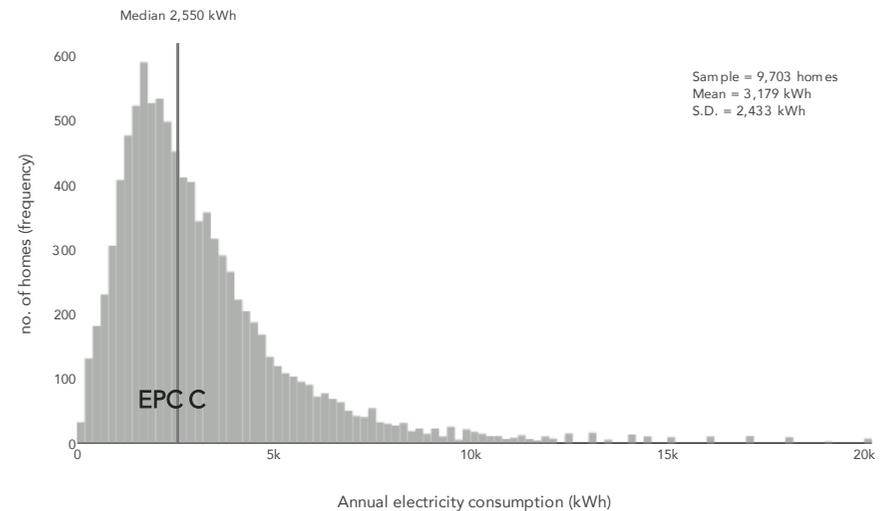
*Electricity consumption for two samples of UK homes from the NEED database, based on EPC band. These are fairly typical distribution for residential electricity meter consumption data. Note the median and modal values, which are close to PHPP calculations shown in following pages.*
