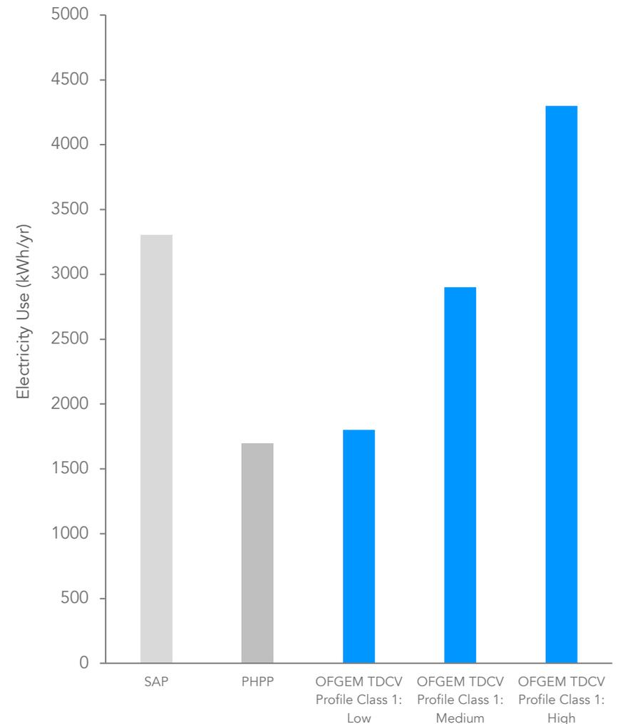
Comparison of SAP and PHPP calculated electricity use with OFGEM Typical Domestic Consumption values for Profile Class 1. It is possible that the domestic TDCVs include a significant amount of non-domestic electricity data, as well as some homes with direct electric heating. This may inflate the consumption values. The OFGEM 25<sup>th</sup> percentile (low TDCV value) aligns well with the PHPP prediction.
