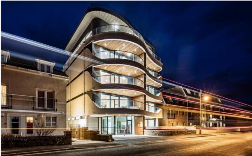
Passivhaus Plus block of flats in Seaton, Devon. Reported an EUI of 25 kWh/m<sup>2</sup>/yr\* and solar generation of 18 kWh/m<sup>2</sup>/yr\* from 2019-2020.
