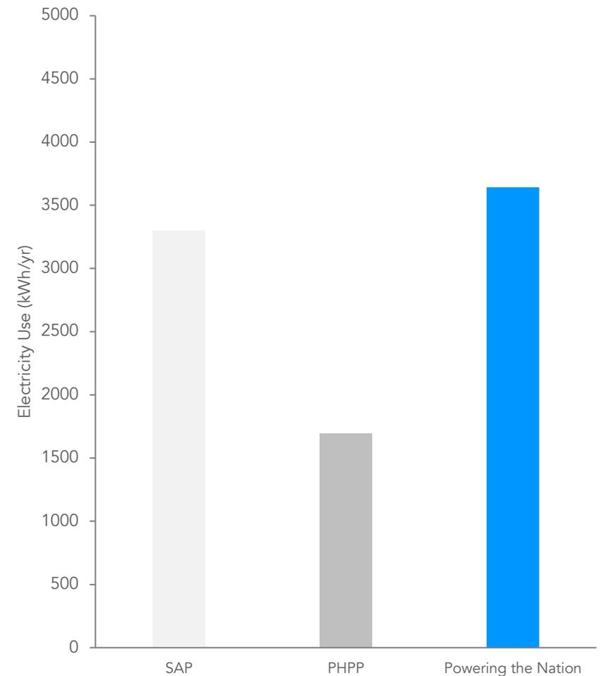
*Comparison of SAP and PHPP calculated electricity use with Powering the Nation Report (2014), based on the Household Electricity Survey from 2010-2011. Electricity use calculated by PHPP is less than half of the mean reported by the study, however much of the difference can be explained by improvements in energy efficiency that are captured in PHPP calculations, and above average levels of electricity use by households selected for the study.*
