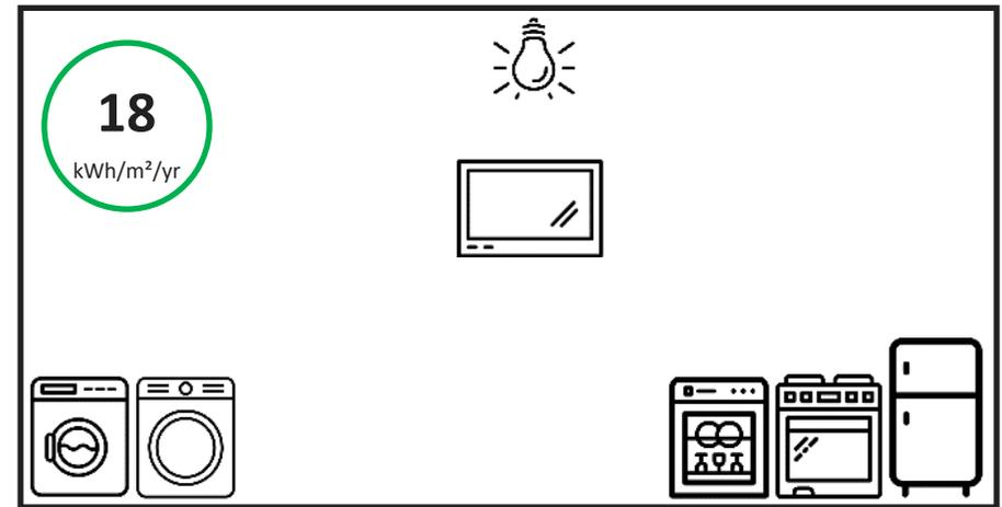
PHPP modelling suggests a typical new build home will use around 1,700 kWh of electricity for appliances, lighting, consumer electronics, and fans and pumps. Divided by the average floor area of 94m<sup>2</sup> GIA, the specific electricity use would be just 18kWh/m<sup>2</sup>/yr.
