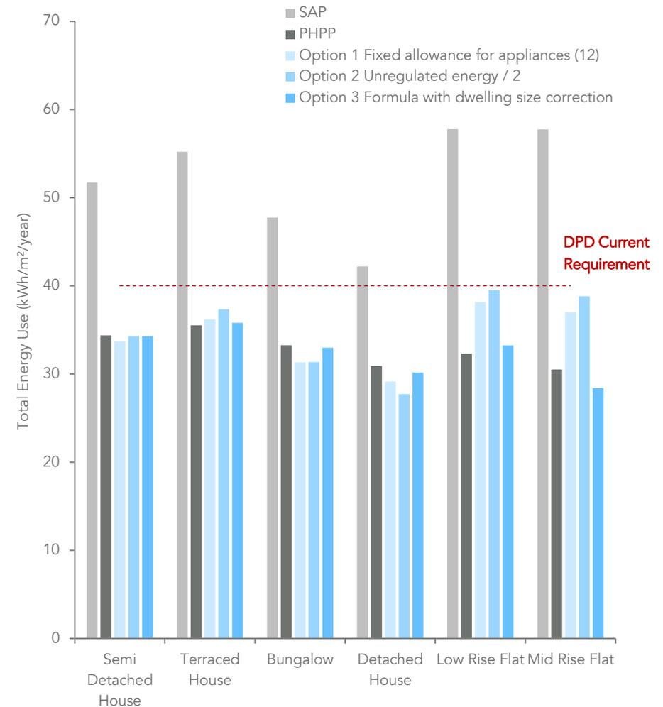
Actual SAP and PHPP total energy use for homes compliant with the current DPD, compared to the results of three different approaches to produce more realistic values from SAP. Options 1 and 2 are simple and do work, though Option 3 produces results more consistent with PHPP calculations. See page 3 for a typical breakdown of dwelling total energy use.
