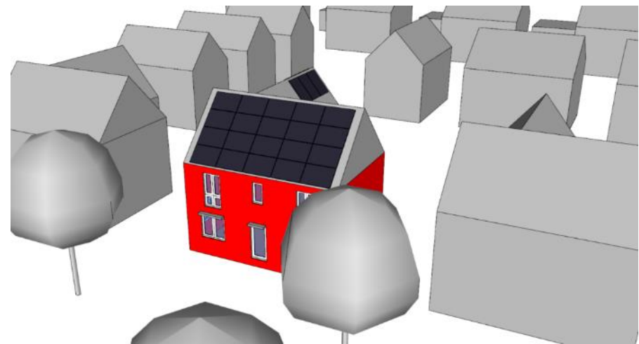
A 3D model of the house and surrounding features was created in DesignPH 2.0.06 and used to calculate solar gains and shading for PHPP.
