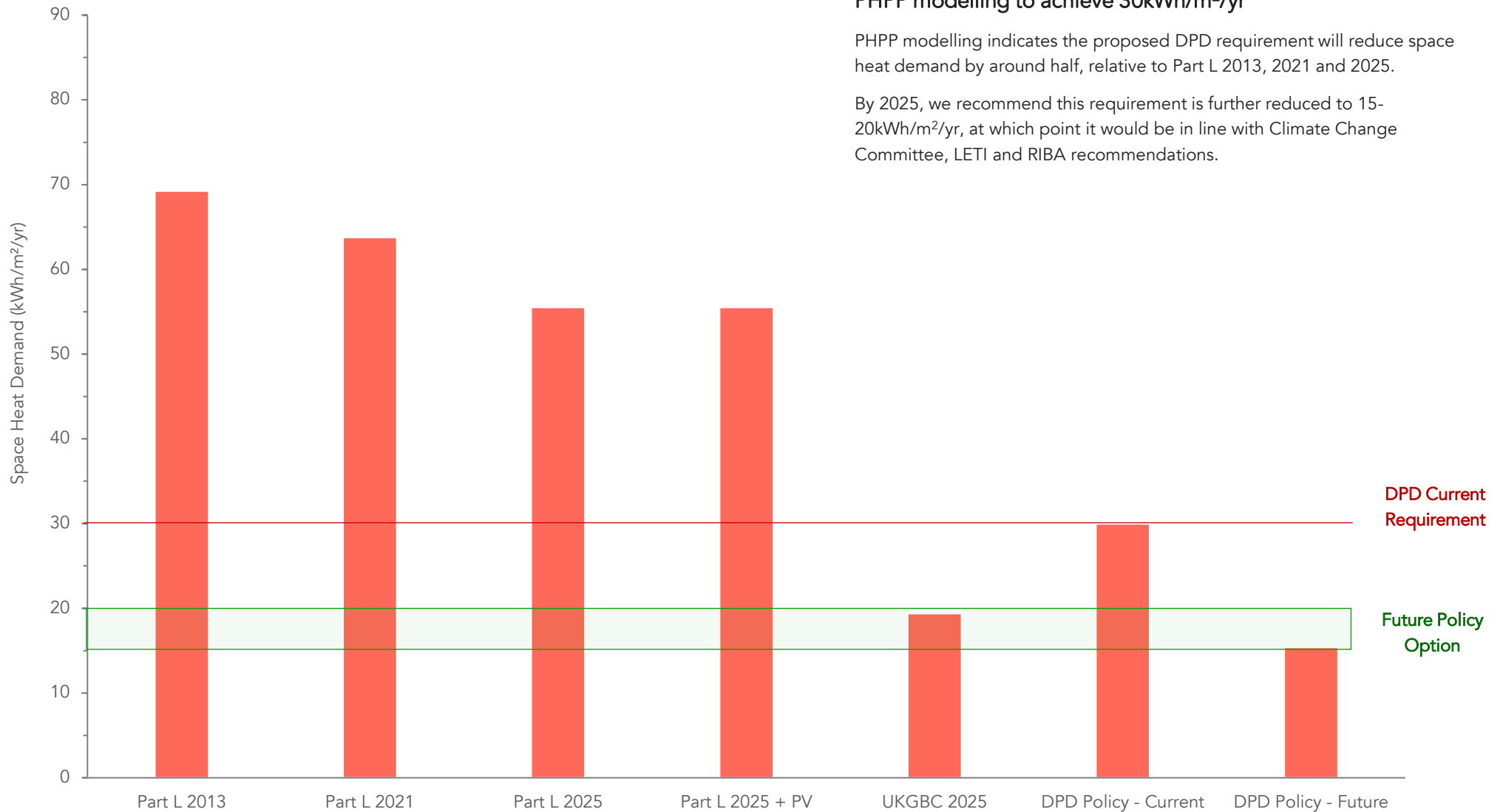
Space heat demand calculated by PHPP 9.6a for each scenario, compared to different policy requirements under consideration.
