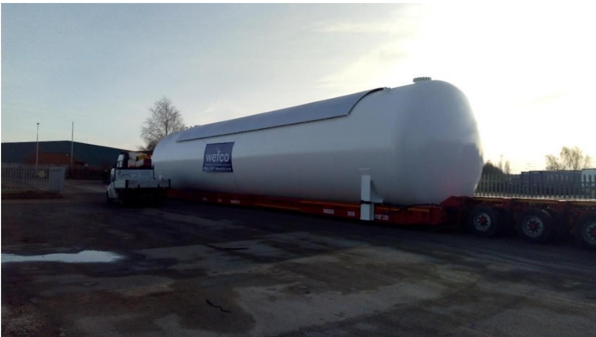
Figure 27: Low pressure hydrogen storage bullet, 25m by 4m diameter.
